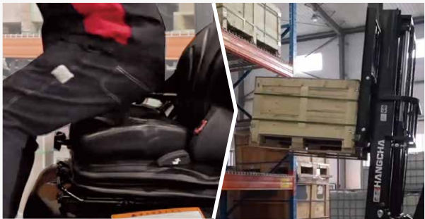
The standard descending lock function (China) can disable the descending function when the driver leaves the seat and enable high safety.
